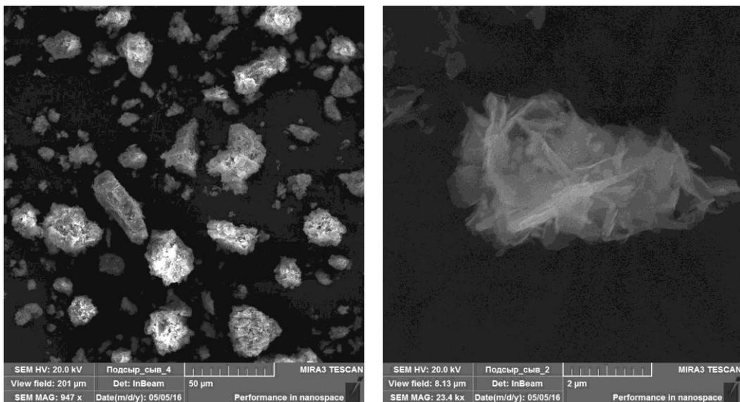
**Fig. 11.** SEM-micro-images of the dry residue of the cheese whey mineralizate.
