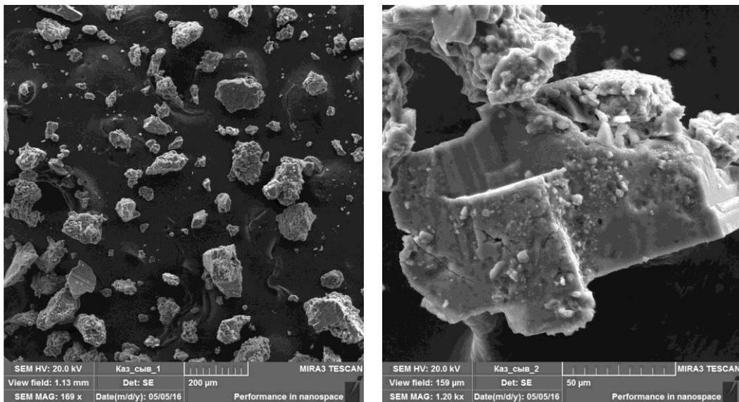
**Fig. 10.** SEM micro-images of the dry residue of casein whey mineralizate.
