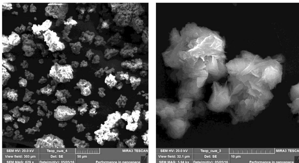
**Fig. 12.** SEM micro-images of the dry residue of curdy whey mineralizate.
