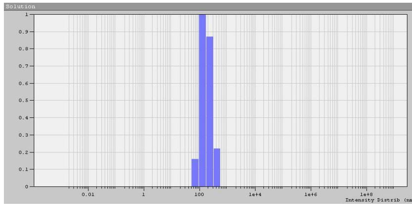
Fig. 5. Histogram of distribution of hydrodynamic radii of particles of the curdy whey disperse phase.
