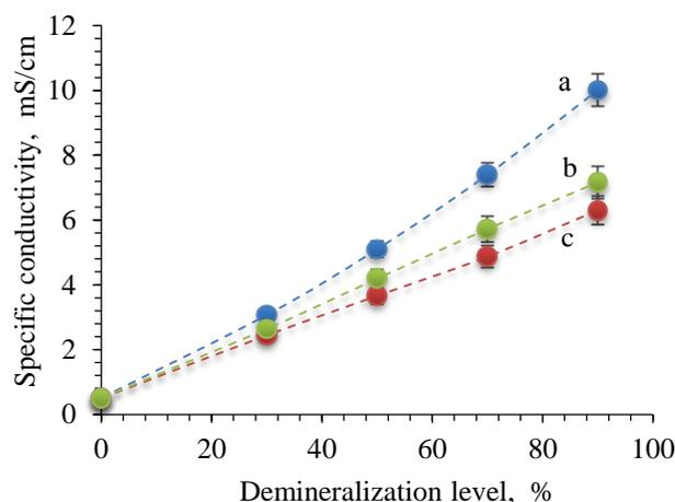
**Fig. 2.** Dependence of specific conductivity of whey mineralizates on the extent of whey demineralization: (a) casein, (b) curdy, (c) cheese.
