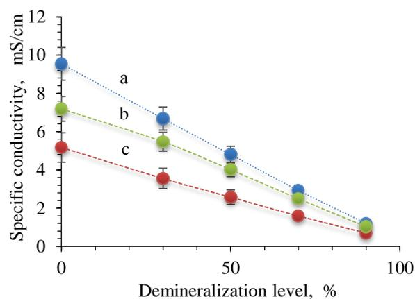
**Fig. 1.** Dependence of specific conductivity of milk whey on the extent of its demineralization: (a) casein, (b) curdy, (c) cheese.
