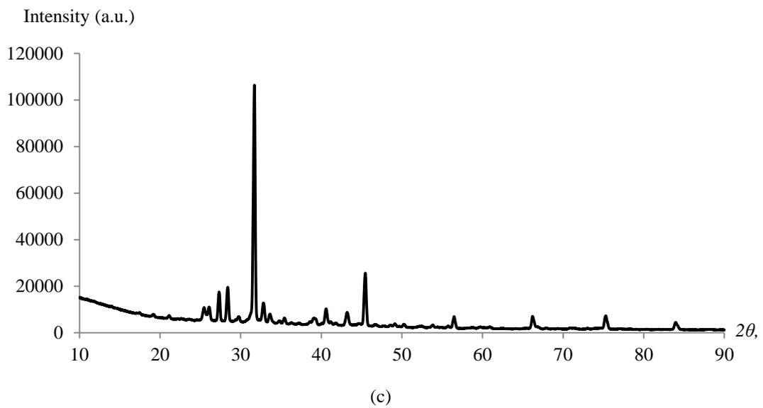
**Fig. 8.** Diffractograms of dry residues of mineralizates of various whey: (a) cheese whey mineralizate; (b) curdy whey mineralizate; (c) casein whey mineralizate.
